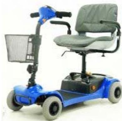
Boot scooters, which would be classified as Class 2, are specifically designed to be compact and easier to fold or dismantle. They can be transported in the boot of a car. Boot scooters differ in weight. You will need to ensure that you, or your carers, can disassemble or fold the scooter, then lift the scooter in and out of the boot and finally reassemble/unfold it at your destination.
